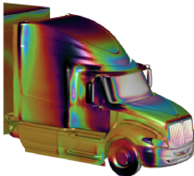
Image of Pressure Distribution over a Semi-Truck Cab: (Image Credit: Simulation results courtesy of Navistar, image Rendered in FieldView)
