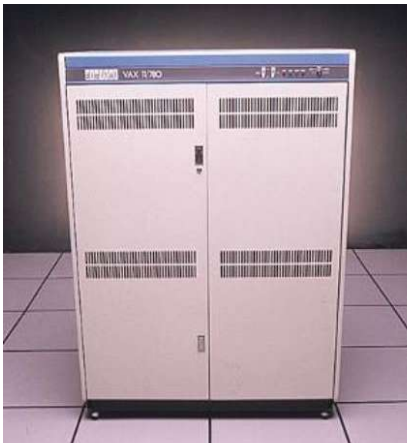
DEC VAX 11/785 One to two 7.2 MHz processor 32-bit word
