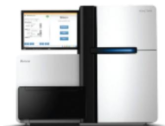
An NGS sequencer converts a DNA sample to images, which are then converted to digital sequence data.
