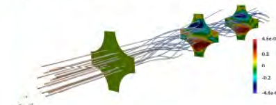
Fluid streamlines downstream of mixing vane
