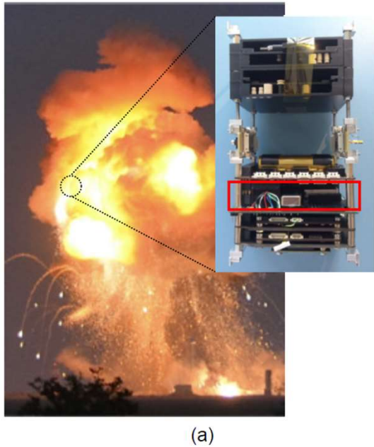
Figure 5.4: (a) GomX-2 CubeSat (without the solar panel) with SPEQS1.1-CS highlighted in red box (b) GomX-2 CubeSat after recovering from the explosion. Images courtesy of GOMspace.
